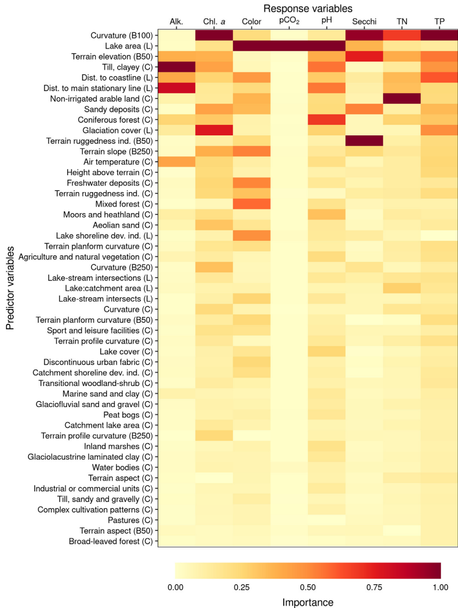
Fig. 4. The permutation variable importance (normalized to 0–1 range with 1 and 0 being the most and least important respectively) of 50 predictor variables calculated using the best performing machine learning model for each of the eight water quality variables. Variables are determined at the levels of the lake (L), catchment (C), and buffer zones (B; e.g., B100 is a 100 m wide buffer zone surrounding the lake).
